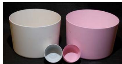
Fig. 4 Net-shaped plasma-spray-formed Y_2O_3 (white) and Er_2O_3 (pink) crucible liners. The large size is 210 mm diameter and the small size is 70 mm diameter. Wall thickness can be varied between 0.5 and 4 mm.
